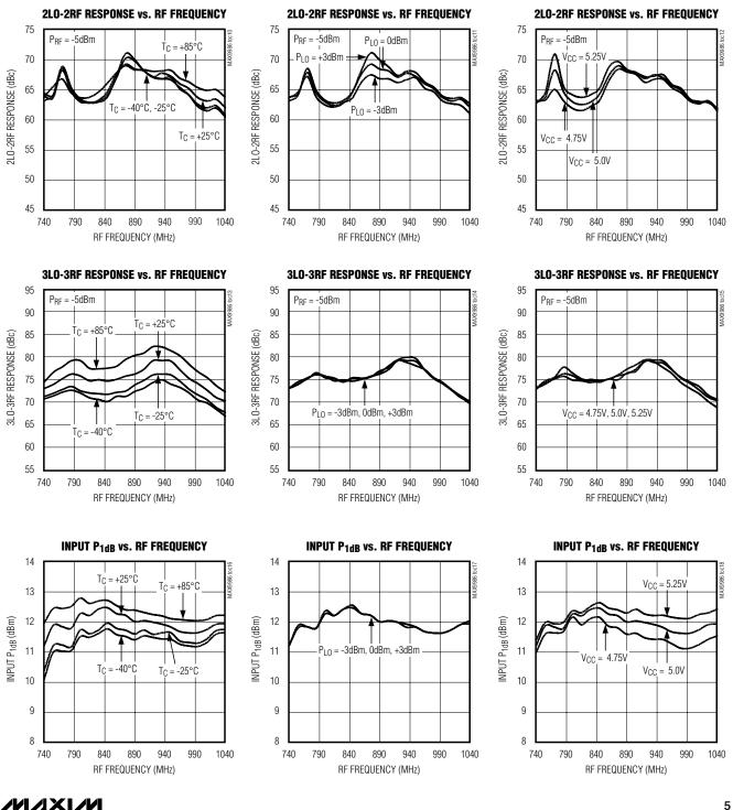
(MAX9986 Typical Application Circuit, V<sub>CC</sub> = +5.0V, P<sub>LO</sub> = 0dBm, P<sub>RF</sub> = -5dBm, f<sub>LO</sub> > f<sub>RF</sub>, f<sub>IF</sub> = 160MHz, unless otherwise noted.)
